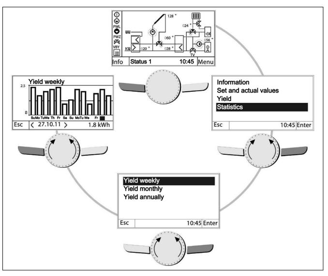
In this Info menu, the solar yields, the heat meters and the flow meters are graphically illustrated.
