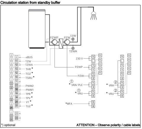
$\textcircled{\sc 0}$  Electrothermic actuator or drive with spring return
