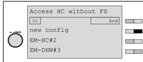
**Menu structure extension module heating circuit (Access HC w.o. FS)**
