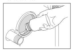
If an external siphon ① is present external to the boiler (e. g. due to the condensate hose):
