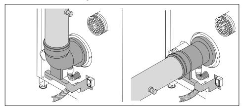
► Install connection set to flue gas connection (see installation and operating instructions WAL-PP).
