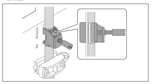
► Connect the cables according to the wiring diagram, in the process pay particular attention to the correct phase location of the voltage supply.
